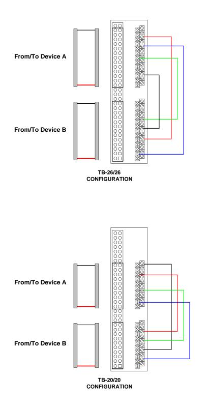
These illustrations show two different Special Order TB-60 boards being used to cross match signals from two different devices connected with same-sized ribbon cables. Many other different combinations are available.
